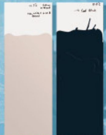
Grey panel is a standard coating. The black panel is coated in Resene Cool Colour technology. The black Resene Cool Colour panel reflects more heat and remains cooler than the standard paint finish on the grey panel.
