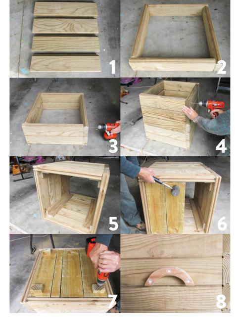
Using the retaining wall timber, cut four lengths 600mm long, then cut a 5° angle at each end. Cut another four lengths 585mm (the final length of your first cut boards), then cut 5° angles at each end.
