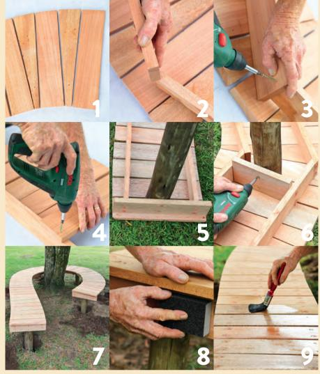
Set out the slats on a flat surface until you get the desired shape. As you go around the curve, every second slat will need to be tapered on both sides to a point approximately 20mm wide. Decide how many slats need to be tapered and cut them to size with a jigsaw. Set them into place.
