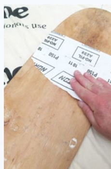
Step three Sand the wood to remove any residue and wipe off any sanding dust with a clean cloth.
