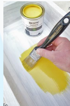
Step four Paint the inside of the cart with two coats of Resene Bright Spark, allowing two hours for each coat to dry.
