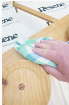
Step two Wipe off any sanding dust with a clean cloth.
